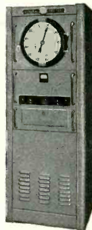
Dewpoint recorder continuously records dewpoint temperature.
