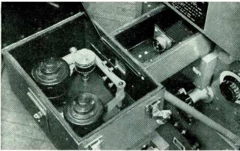
FIG. 3—Two-kilocycle marking lines from master oscillator (right) are projected through optical system to 35-mm film strip of oscillator under test which runs in a light-tight box shown here with cover removed
