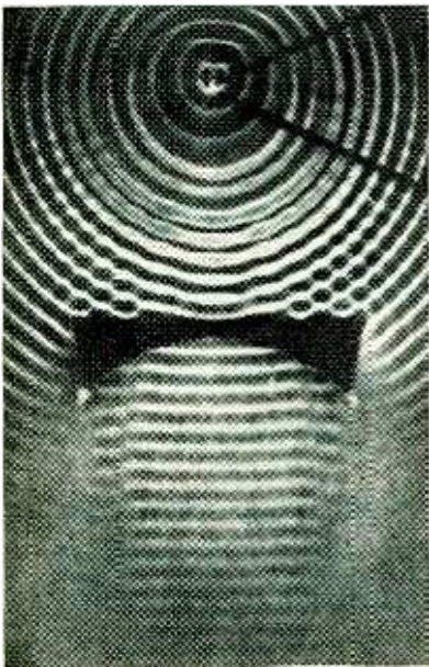
FIG. 2—Typical problems suitable for ripple-tank study include the effects of waveguide lenses on phase fronts
