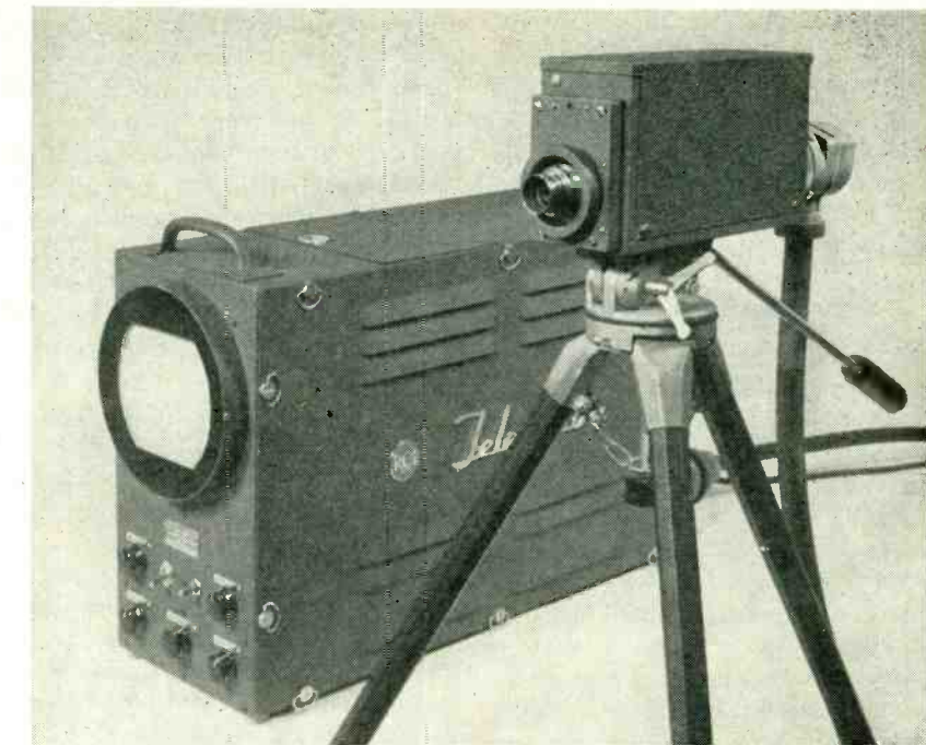
Miniature television camera employing the vidicon pickup tube 6 , with standard image-orthicon camera in background
