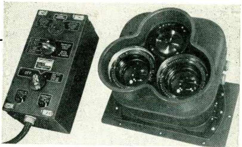
Assembled lens turret beside control box that contains all the electron tubes
