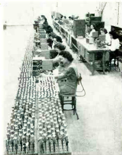
Small forest of electron guns moves along production line at RCA's new Marion, Ind., plant
