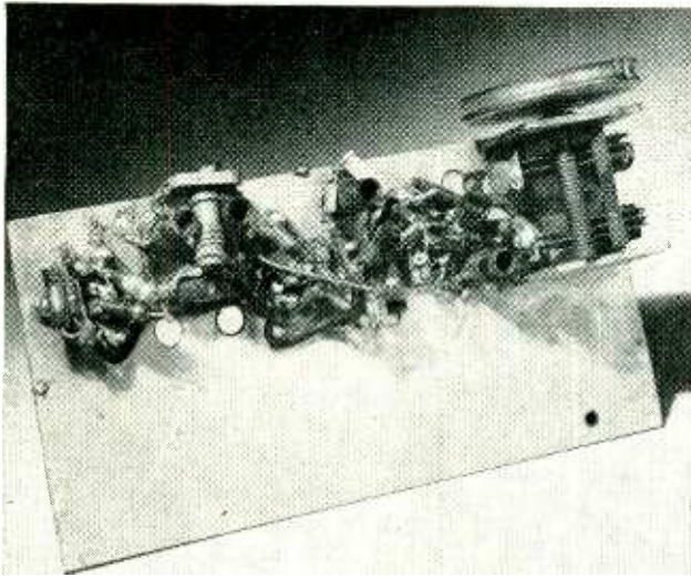
Coils and trimmers between sockets are part of low-band bridged-T coupling network. Circuit for chassis shown is Fig. 4A
