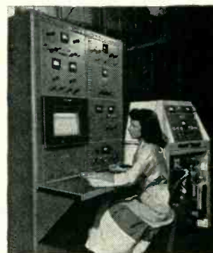
G-E mass spectrometer gives direct readings—no waiting for photographs.
