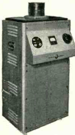
Dewpoint recorder continuously records dewpoint temperature.
