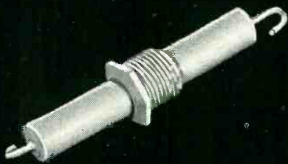
16 Special feed-thru by-pass capacitor.
