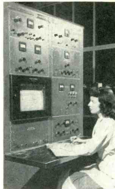
Panel of new G-E mass spectrometer showing Elektronik strip chart recorder
