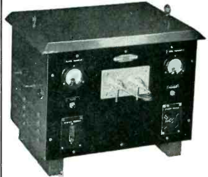
Vertical and Horizontal Blocking Oscillator. Above Chassis mounting
